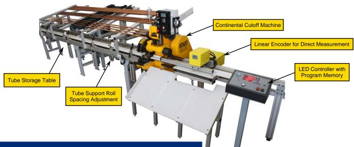
Programmable, automatic tube feeders are available for all Continental pipe and tube cut-off machines. From simple "one-stick-at-a-time" feeders to complete tube bundle to cut parts systems.
